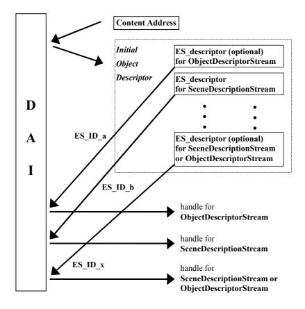
Figure 8 — Requesting stream delivery through the DAI
