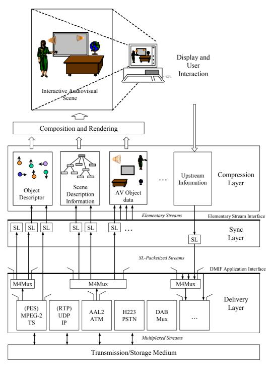
Figure 1 — The ISO/IEC 14496 Terminal Architecture
