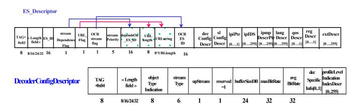
When present, the decSpecificInfo descriptor is an opaque descriptor (tag=0x05), configured according to the ObjectDescriptorID and to the streamType.
