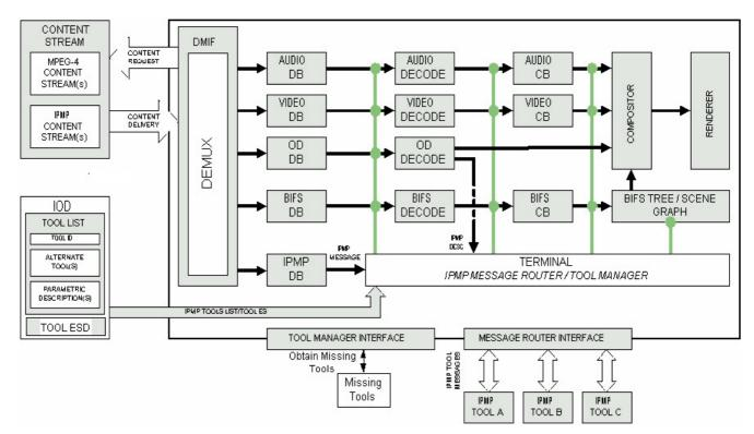
Figure 9 — IPMP system in the ISO/IEC 14496 terminal architecture
