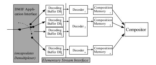
Figure 2 — Systems Decoder Model
