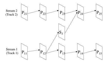
Figure 3 — Stream switching
