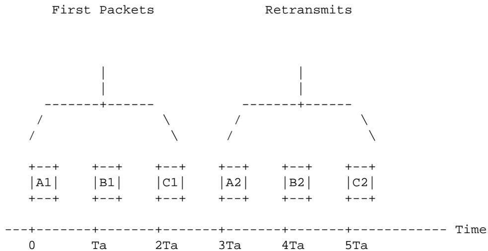
In this picture, there are three transactions that will be sent (for example, in the case of candidate gathering, there are three host candidate/STUN server pairs). These are transactions A, B, and C. The retransmit timer is set so that the first retransmission on the first transaction (packet A2) is sent at time 3Ta.
