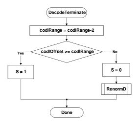
Figure 9-7 - Flowchart of decoding a decision before termination
