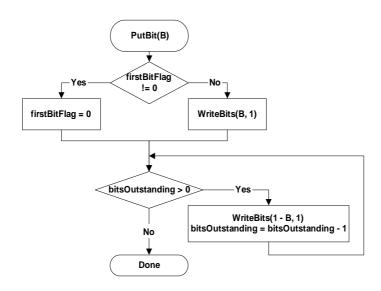
Figure 9-11 – Flowchart of putting bit
