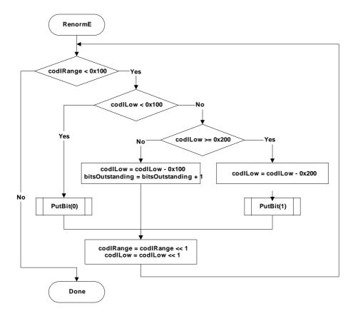
Figure 9-10 - Flowchart of renormalization in the encoder
