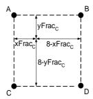
Figure 8-6 – Fractional sample position dependent variables in chroma interpolation and surrounding integer position samples A, B, C, and D.
