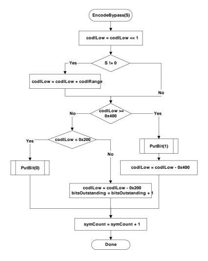
Figure 9-12 - Flowchart of encoding bypass
