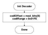
Figure 9-2 – Flowchart of initialisation of the decoding engine
