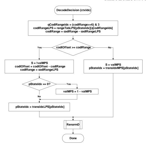
Figure 9-4 - Flowchart for decoding a decision
