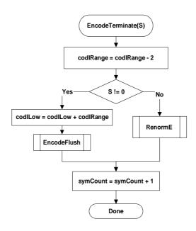
Figure 9-13 - Flowchart of encoding a decision before termination
