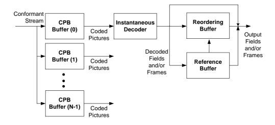
Figure C-2 - HRD buffer model
