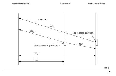
Figure 8-3 A direct-mode B partition has two derived motion vectors (mvL0, mvL1) pointing to two reference pictures referred by refIdxL1. [Ed. Note(YK): In the figure, MV, MV0, and MV1 should be changed to mvCol, mvL0, and mvL1, respectively.]
