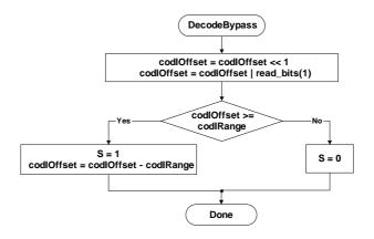
Figure 9-6 – Flowchart of bypass decoding process
