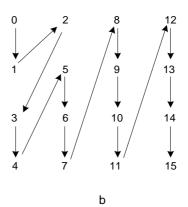
Figure 8-9 – a) Zig-zag scan. b) Field scan
