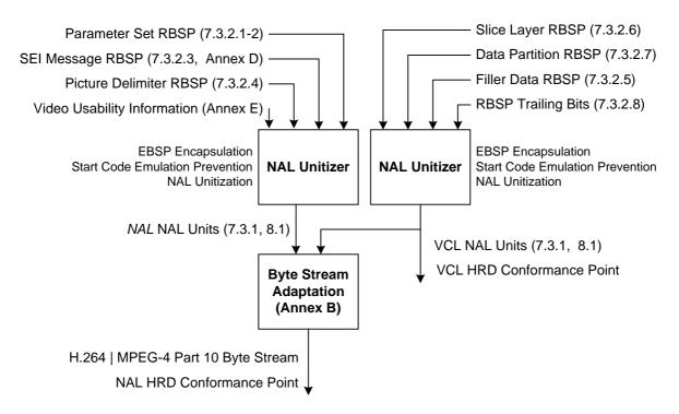
Figure C-1 – Structure of byte streams and NAL unit streams and HRD conformance points
