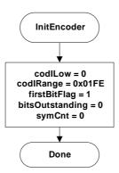
Figure 9-8 – Flowchart of initialisation of the encoding engine
