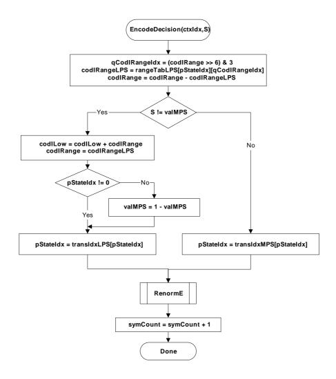
Figure 9-9 - Flowchart for encoding a decision
