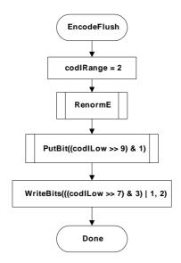
Figure 9-14 – Flowchart of flushing at termination
