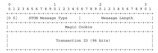
Figure 2: Format of STUN Message Header
